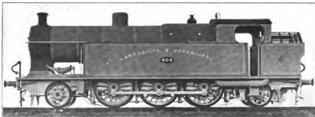
Fig. 5038. Ten-Wheel, Six-Coupled Tank Locomotive with Radial Axle Boxes. Lancashire & Yorkshire. Cylinders 19 in. x 26 in.; Working Steam Pressure 180 lbs. per sq. in.; Total Heating Surface 2,038.64 sq. ft.; Diameter of Drivers 68 in.; Weight on Drivers 127,730 lbs.; Total Weight 184,600 lbs.
